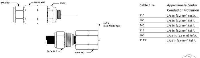
As a final check on both coring depth and center conductor length, install the main nut onto the cable. The center conductor will protrude 1/16" to 1/8" past the end of the main nut. Use the reference table to verify correct center conductor length according to each cable size. The center conductor once cut to length should protrude from end of main nut surface [Ref A].
